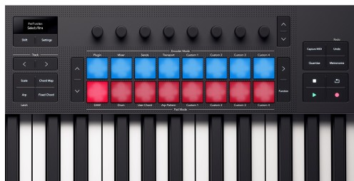
The Launchkey's pads in Logic's Select/Arm mode.
