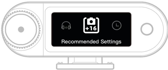
The value "+16" indicates the current camera RX output gain level.
