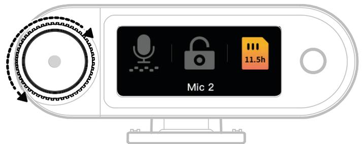
1. When the Mic is connected to the Camera RX, tap the red-framed area on the touchscreen to enter the shortcut menu.
