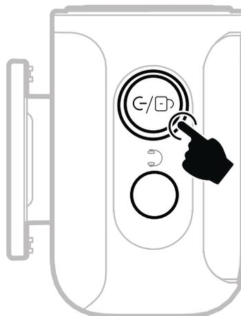
To pair the Mic(s), power off the camera RX and press and hold the pairing button for 6 seconds.
