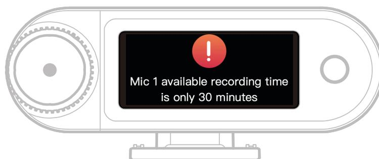
When the Mic's internal recording storage has less than 30 minutes remaining, the Camera RX will display a warning: "Mic1 available recording time is only 30 minutes." Once the storage is full, the Mic will continue recording by overwriting the oldest files in a rolling recording mode. You can format the memory via the Camera RX or delete recordings by connecting to a computer.
