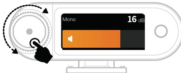
\*After configuring the Recommended Settings, if the audio level is perceived as too loud or too quiet, adjust the RX output gain accordingly using the control knob.
