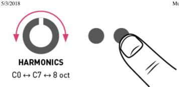
After having turned the **HARMONICS**, **TIMBRE** or **MORPH** knob to adjust a setting, the position of the knob might no longer match the original value of the corresponding parameter. When this happens, the response curve of the knob is modified to account for this discrepancy, until the position of the knob and the parameter perfectly line up again!
