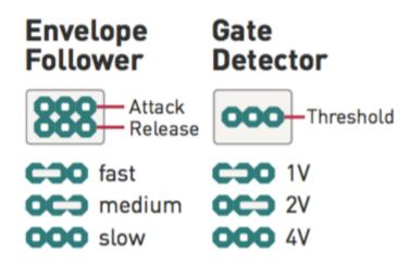
The last setting, corresponding to the longest time or higher voltge, is obtained by removing the jumper.
