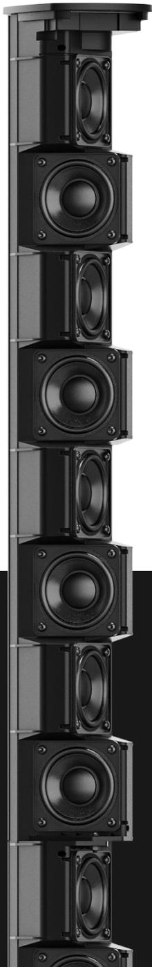
The Bose L1 Pro series incorporates line array technology that provides advantages compared to a traditional point source portable PA loudspeaker. In general, line array technology provides more targeted audience coverage as it acoustically aims its sound energy to the intended listening area and away from non-intended areas like the ceiling or floors.
