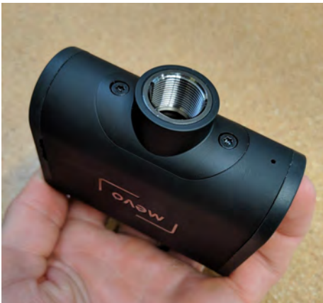
1/4"-20 UNC tripod thread
