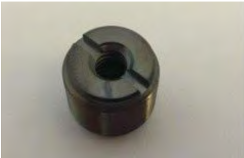
1/4"-20 UNC tripod thread
